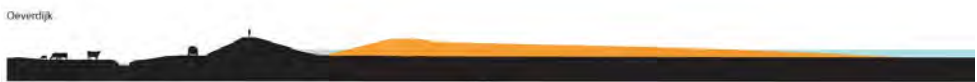
Figure 5.4 Cross-section of a Basic Flood Protection shore dike (Van der Linde et al., 2012)
