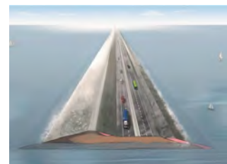
Figure 6.4 Afsluitdijk overflow-resistant dam design
